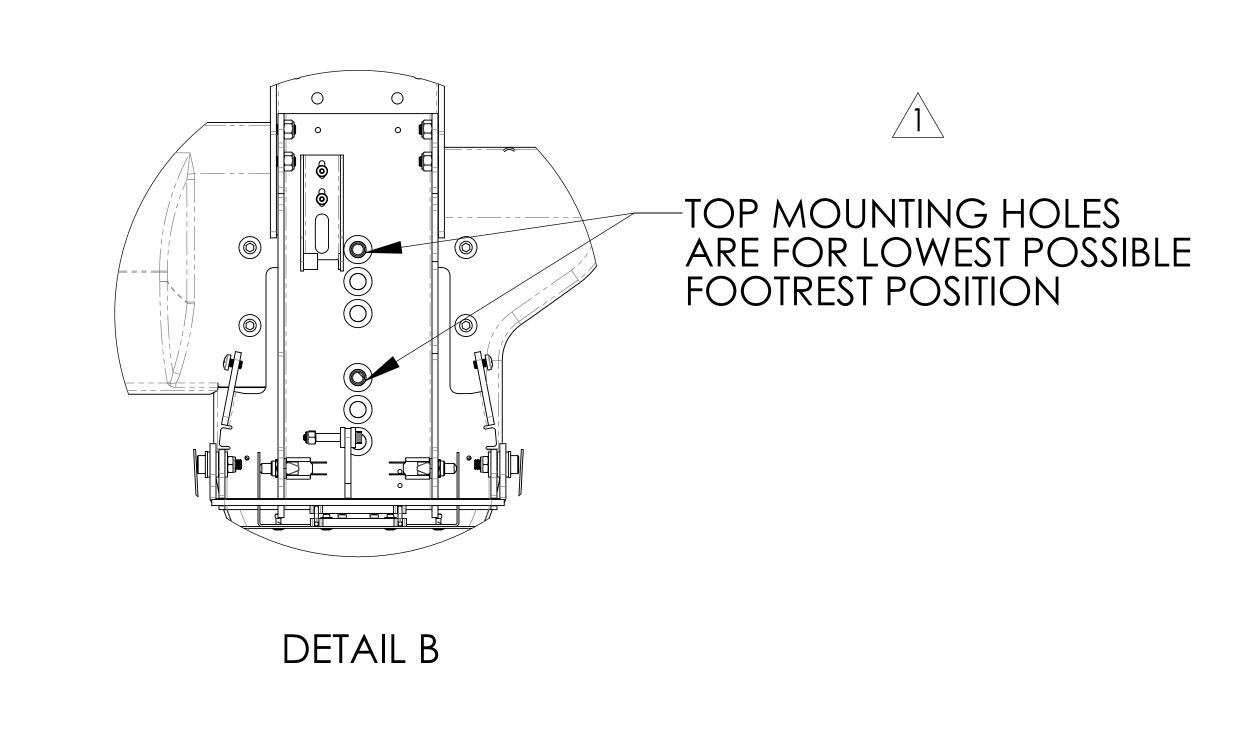
NOTE: WHEN THE BOTTOM FOOTREST MOUNTING HOLES ARE USED, THE SEAT WILL BE IN ITS HIGHEST POSITION.
