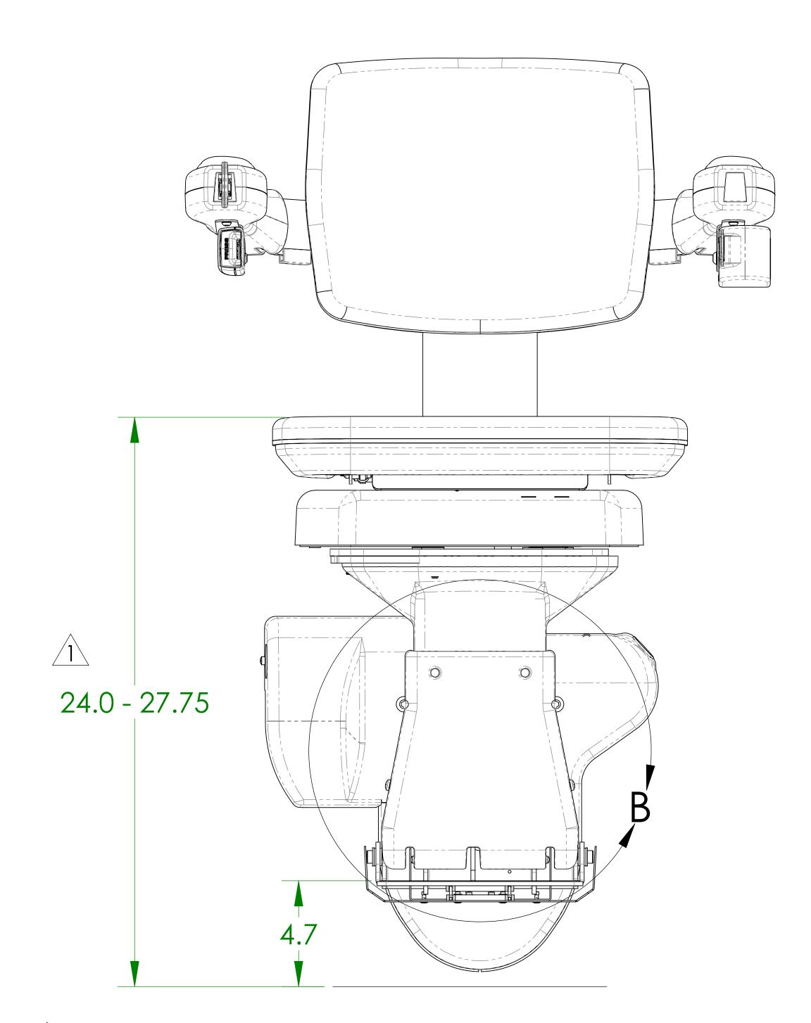
POWER SWIVEL SEAT AND POWER FOLDING FOOTREST (USES TOP MOUNTING HOLES, LOWEST USABLE FOOTREST POSITION ON CRE-2110) (SEE DETAIL B)
